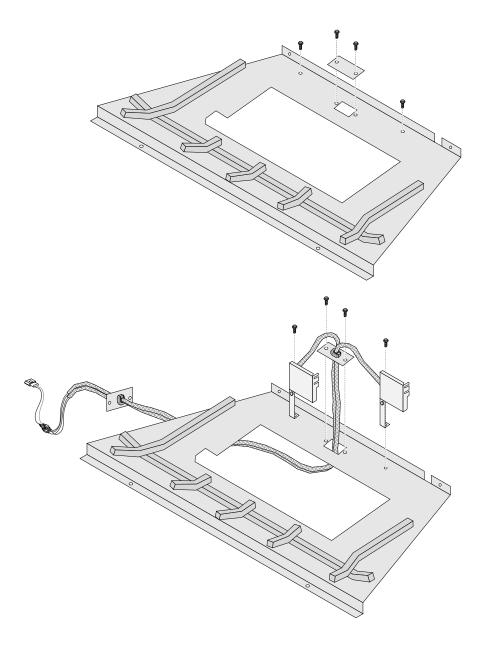
Remove the cover plate and two screws on the firebox floor. The cover plate may be discarded (keep the screws for accent light attachment).
